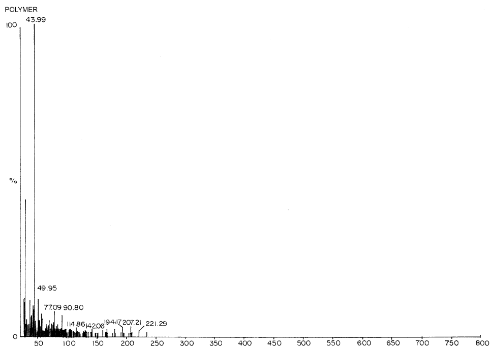
Figure 10. The mass spectrum of polymer with a 70 eV electron impact.
